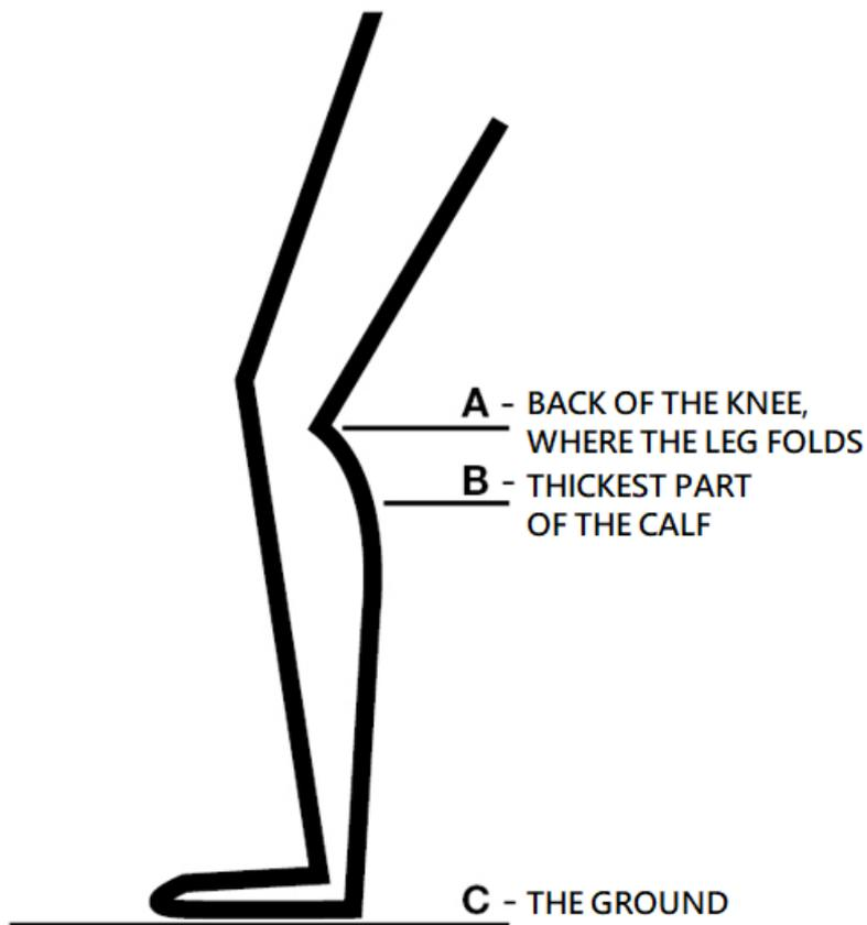
Measure with a tape measure on the leg between points A and C and compare with the table above which stilt should be used.
