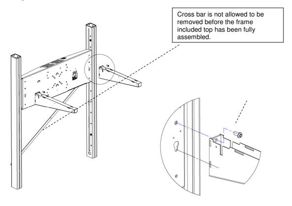
**b)** Mount four fixing brackets for top and attach three lead holders with screws.
