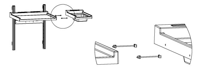
b) Make two ø8 mm holes in both top and sink as shown in drawing. Holes to be used with the fixing bolts.
