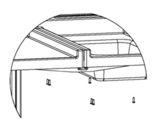
The crack between the two tops can be sealed with sealant. Be sure to clean the surface with a gentle household cleanser prior to sealing. Tops are made of ABS.
