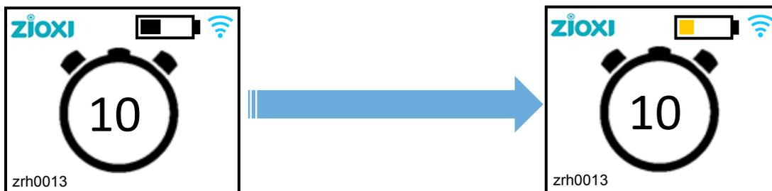
Once the battery gauge symbol changes from Black to Amber it is advisable to recharge the powerHub. Once the battery gauge changes to a single Red bar then the powerHub should be re-charged immediately.
