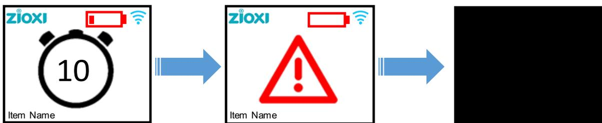
If the powerHub is left for a further period of time without re-charging then to protect it's batteries it will automatically turn off power to the powerHub sockets, display a red warning
