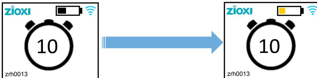
Once the battery gauge symbol changes from Black to Amber it is advisable to recharge the powerHub at the next convenient opportunity. Once the battery gauge changes to a single Red bar then the powerHub should be re-charged immediately.
