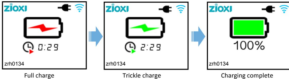
The charging mode will automatically change between the 3 modes as each phase of charging is completed. The length of time required for a full charge from a fully depleted battery will vary depending on the powerHub capacity but will typically be 12 to 16 hours. **zioxi** onView can also be used to remotely monitor the Charging status.
