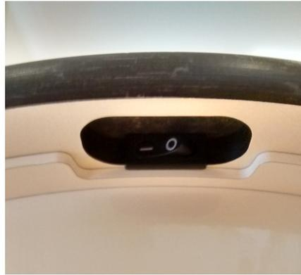
Toggle this switch to the on position so the powerHub screen comes on. This on / off switch can be used to turn off the powerHub at any point (eg. during holiday periods) and may be useful if the powerHub needs to be “re-booted”.
