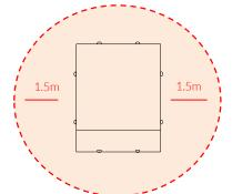
Install Instrument with 1.5m free space (from widest point) around it.
