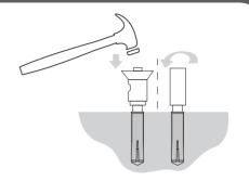
Q Use the HILTI HSD-G M12x50 or HSD-M M12x50 setting tool to widen the bottom of the anchors.
