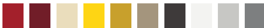
RAL3002 Carmine red ≈2570-Y90R RAL 3004 Purple red ≈5040-R RAL1015 Light ivory ≈1010-Y20R RAL1018 Zinc yellow ≈0570-Y RAL 1005 Honey yellow ≈2070-Y10R RAL 1019 Grey beige ≈4010-Y30R RAL8019 Grey brown ≈9000-N RAL9016 Traffic white ≈0502-G50Y RAL7047 Telegrey 4 ≈2000-N RAL7037 Dusty grey ≈5500-N
